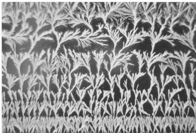
Fig. 10 Periodic tree-like morphology of \text{PbCl}_2 in PVA film. Gel: 3.5/250 inner electrolyte: 0.03 M \text{Pb}(\text{NO}_3)_2 , outer electrolyte: 1.0 M NaCl
